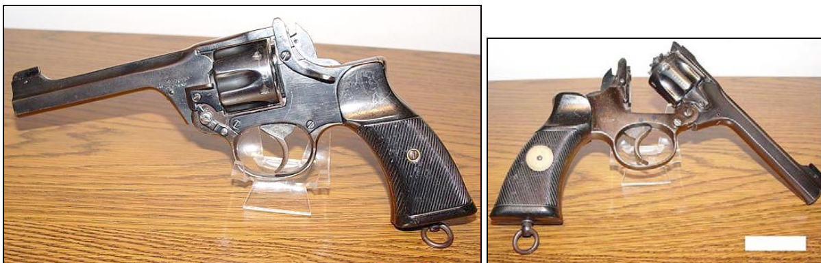
FIGURE 14: The Webley MkV double action .38 calibre revolver.
